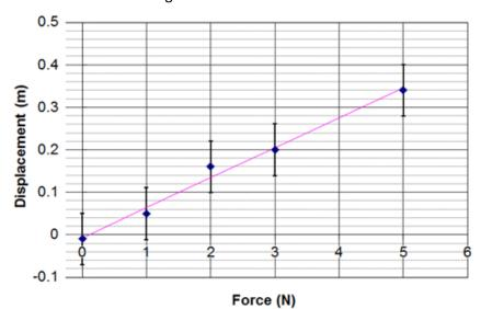
We calculate the slope using the actual rise ( $\Delta y$ ) and run ( $\Delta x$ ) from the graph. The best-fit line goes through the points (0, 0) and (3.0, 0.21). From these points, we would calculate the slope as:
