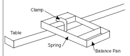
The balance pan is pulled to one side, causing it to oscillate. The balance is calibrated with objects of known mass, and the period of oscillation is then used to determine the mass of the unknown object.
