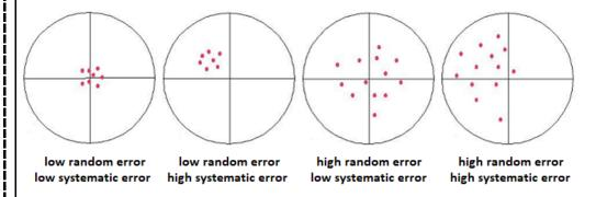
The first set has *low random error* because the points are close to each other. It has *low systematic error* because the points are approximately equally distributed about the expected value.
