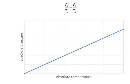
Note that at absolute zero, gas molecules do not exert any pressure on the walls of the container.
