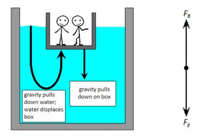
If the object floats, it reaches its equilibrium when the weight of the object and the weight of the water that was displaced (and is trying to displace the object) are equal.
