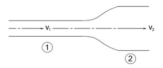
In order to squeeze the same volume of fluid through a narrower opening, the fluid needs to flow faster. Because Av must be constant, the cross-sectional area times the velocity in one section of the pipe must be the same as the cross-sectional velocity in the other section.
