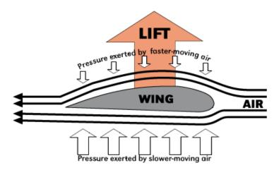
(Of course, most of an airplane's lift comes from the fact that the wing is inclined with an angle of attack relative to its direction of motion, an application of Newton's third law.)
