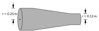
If the fluid in the pipe is flowing at  $5.2\,\frac{m}{s}$  at the inlet, then how fast is it flowing at the outlet?
