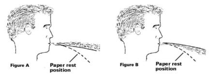
The air moving across the top of the paper causes a decrease in pressure, which causes the paper to lift.
