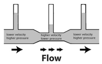
This pipe is horizontal, which means h is constant; therefore  $\rho gh$  is constant. This means that if  $\frac{1}{2}\rho v^2$  increases, then pressure (P) must decrease so that  $P_{ext} + \rho gh + \frac{1}{2}\rho v^2 = \text{constant}$ .
