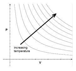
As temperature increases, the isotherm moves farther away from the origin.
