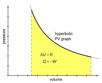
$$\frac{P_1V_1}{f_1} = \frac{P_2V_2}{f_2} \quad \rightarrow \quad P_1V_1 = P_2V_2$$
