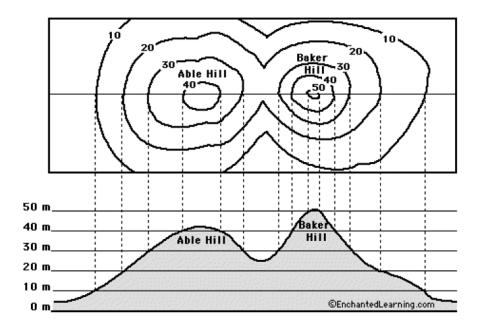
The contour map (top) is a view from above. Each contour line connects points that have the same elevation.
