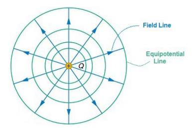
Notice that the equipotential lines are perpendicular to the field lines. As you travel along a field line, the electric potential becomes continuously less positive or more negative. The equipotential lines are the mileposts that show what the electric potential is at that point.
