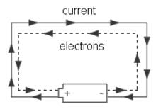
This means that electric current "travels" in the <u>opposite</u> direction from the electrons. We will use conventional current (pretending that positive particles are flowing through the circuit) throughout this course.
