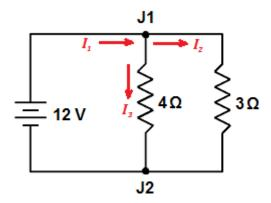
The junction rule tells us that the current flowing into junction J1 must equal the current flowing out. If we assume current  $I_1$  flows into the junction, and currents  $I_2$ and  $I_3$  flow out of it, then  $I_1 = I_2 + I_3$ .
