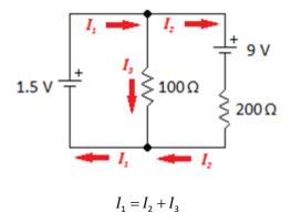
By closer inspection, we can see that the direction for  $I_2$  is probably going to be wrong. This means we expect that  $I_2$  will come out to a negative number.
