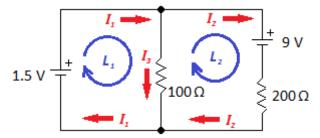
chosen for current. The loop direction is simply the order in which we inspect each element. The numbers will be determined by the direction we chose for current.
