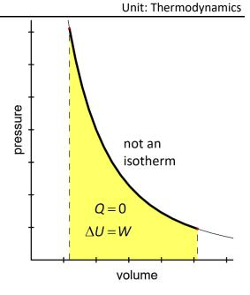
Note that adiabatic expansion (sudden increase in volume without time for heat transfer) results in a decrease in temperature, and adiabatic compression (sudden decrease in volume without time for heat transfer) results in an increase in temperature.
