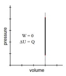
Because the volume is not changing, there is no way for the gas to displace anything. (Recall from Physics 1 that  $W = \vec{F} \cdot \vec{d}$ .) If there is no displacement, there is no work, which means W = 0.
