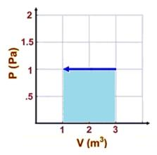
The pressure is P = 1 Pa, and the change in volume is  $\Delta V = -2$  m<sup>3</sup>. Because pressure is constant, we can use  $W = -P\Delta V = -(1)(-2) = +2 J$ .
