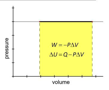
Isobaric changes involve changes in both Q and W, because to change the volume of a gas while keeping pressure constant, you need to add or remove heat, but the resulting change in volume means that work is being done.
