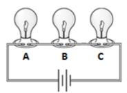
In a series circuit, all of the current flows through every component, one after another. If the current is interrupted anywhere in the circuit, no current will flow. For example, in the following series circuit, if any of the light bulbs A, B, or C is removed, no current can flow and none of the light bulbs will be illuminated.
