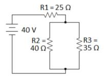
Because the circuit has series and parallel sections, we cannot simply use the series and parallel rules across the entire table.
