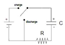
When this happens, the capacitor discharges (loses its charge). The capacitor acts as a temporary voltage source, and current temporarily flows out of the capacitor through the resistor.
