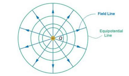
Notice that the equipotential lines are perpendicular to the field lines. As you travel along a field line, the electric potential becomes continuously less positive or more negative. The equipotential lines are the mileposts that show what the electric potential is at that point.
