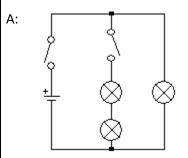
Note that no sensible person would intentionally wire a circuit this way. It would make much more sense to have the second switch on the branch with the one light bulb, so you could turn off either branch separately or both branches by opening both switches. This is an example of a strange circuit that a physics teacher would use to make sure you really can follow exactly what the question is asking!
