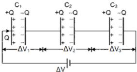
Note that the segment of the circuit that goes from the right side of  $C_1$  to the left side of  $C_2$  is isolated from the rest of the circuit. Current does not flow through a capacitor, which means charges cannot enter or leave this segment. Because charge is conserved (electrical charges cannot be created or destroyed), this means the negative charge on  $C_1$  (which is  $-Q_1$ ) must equal the positive charge on  $C_2$  (which is  $+Q_2$ ).
