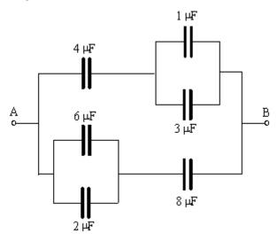
First we would add the capacitances in parallel. On top,  $3 \mu F + 1 \mu F = 4 \mu F$ . On the bottom,  $6\,\mu\text{F} + 2\,\mu\text{F} = 8\,\mu\text{F}$  . This gives the following equivalent circuit:
