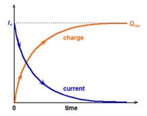
(Note that the graphs are not to scale; the y-axis scale and units are necessarily different for charge and current.)
