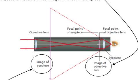
The image from the objective lens is then refracted by the eyepiece. The eyepiece creates a much larger virtual image, which is what the eye sees.
