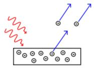
The photoelectric effect requires light with a sufficiently high frequency, because the frequency of the light is related to the amount of energy it carries. The energy of the photons needs to be above a certain threshold frequency in order to have enough energy to ionize the atom.
