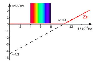
The maximum kinetic energy of the emitted electron is equal to Planck's constant times the difference between the frequency of incident light (f) and the minimum threshold frequency of the element  $(f_o)$ :
