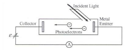
In the above schematic, two metal plates are placed in a vacuum chamber. Monochromatic light (light of only one frequency) is shone onto the metal emitter, causing electrons to be emitted.
