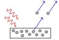
The photoelectric effect requires light with a sufficiently high frequency, because the frequency of the light is related to the amount of energy it carries. The energy of the photons needs to be above a certain threshold frequency in order to have enough energy to ionize the atom.
