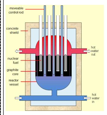
The fuel is the radioactive material (such as <sup>235</sup>U) that is undergoing fission. The graphite in the core of the reactor is used to absorb some of the neutrons. The moveable control rods are adjusted so they can absorb some or all of the remaining neutrons as desired. If the control rods are all the way down, all of the neutrons are absorbed and no heating occurs. When the reactor is in operation, the control rods are raised just enough to make the reaction proceed at the desired rate.
