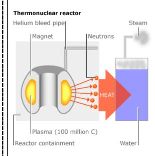
The major challenge in building nuclear fusion reactors is the high temperatures produced—on the order of  $10^6 - 10^9$  °C. In a tokamak fusion reactor, the starting materials are heated until they become plasma—a sea of highly charged ions and electrons. The highly charged plasma is kept away from the sides by powerful electromagnets.
